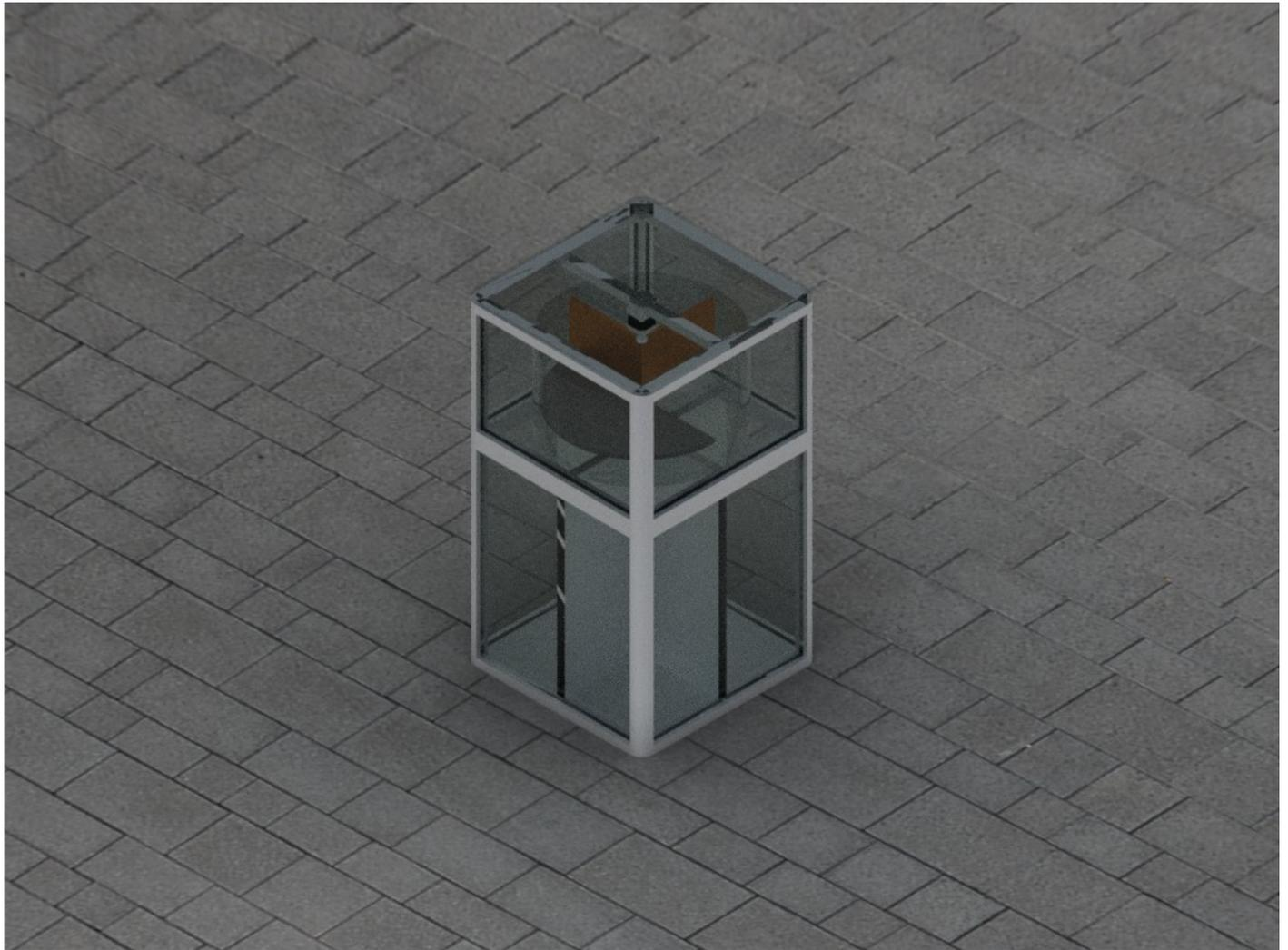
Uses about 75% of space for storage, however cannot handle more than one piece of waste at a time
