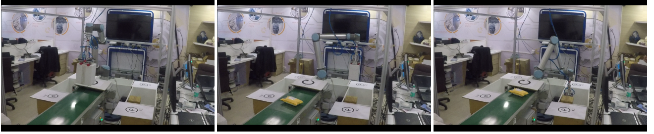
Figure 1: Prototype created in the lab. The conveyor belt brings single-sorted parcels with regular spacing. Demonstration of one pick and place cycle is shown, from left to right (a) Picking the parcel from the conveyor belt (b) Searching for the placement location (c) Placing the parcel inside the container.
